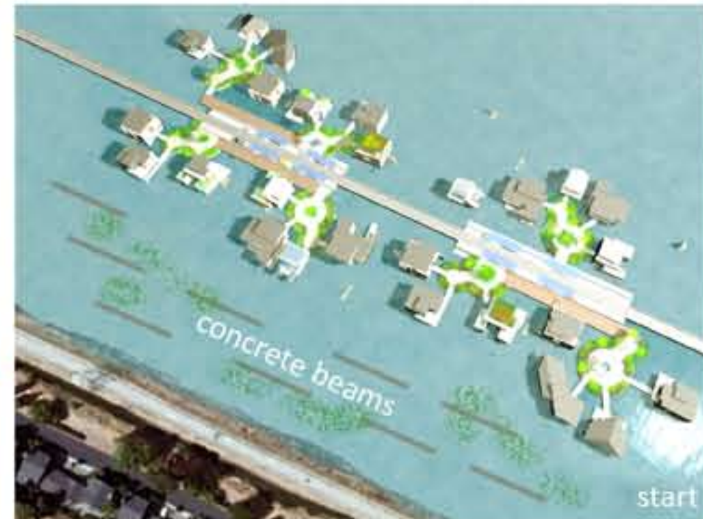
Figure 3: The floating community creates a quiet zone where sediments can settle. Recycled concrete beams accelerate this process
